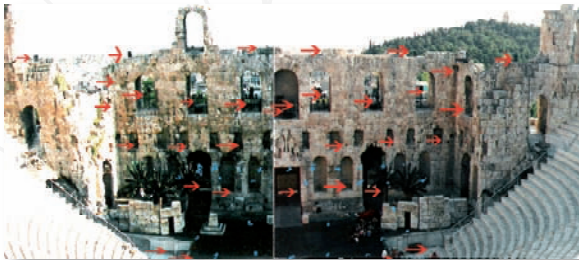
Electroacoustic enhancement at Herodeion Teater with 28 mikrophones (blue) and 32 laoudspeakers (red)
